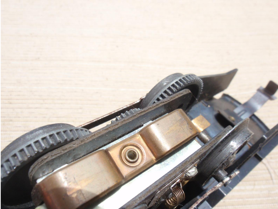
Marx Steam Loco with Single Reduction Bottom View – note that the gears come all the way to the edge of the flange. Some call this the ‘thick flange version’ because it will not work through some brands of switches or crossings. The guard rails interfere.
